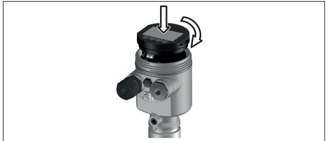
Fig. 20: Installing the display and adjustment module in the electronics compartment of the single chamber housing
