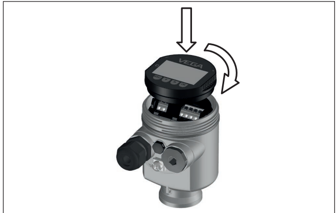
Fig. 37: Installing the display and adjustment module in the electronics compartment of the single chamber housing
